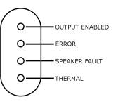
Any flashing lights after the initial start-up phase indicates that a possible fault has been detected. In this case you should note the indicator status and then immediately switch-off the amplifier and consult the following table to check what steps need to be taken.
