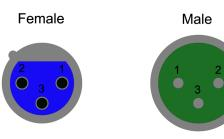
By convention, the two signals are referred to as the positive phase (sometimes referred to as 'hot') and the negative phase ('cold').
