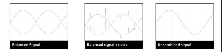
Now when the two wave forms are recombined (by subtracting one from the other) the noise cancels itself out, leaving the original, noise-free signal.
