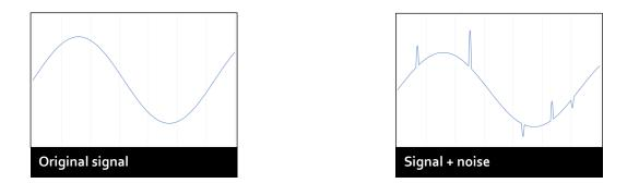
Unfortunately, once the signal has become corrupted with noise, there is no method of removing this noise without further damaging the original signal.
